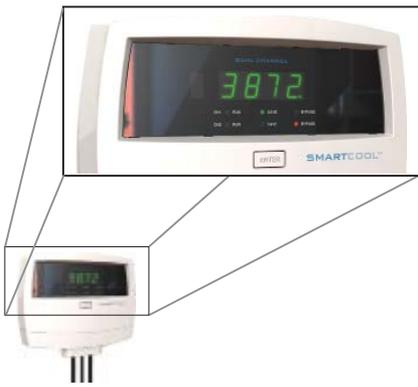
There are 4 displayed digits, but values up to 65000 are displayed. For values up to 9,999 the format is d.ddd and for values above 9,999 the format is dd.dd. Hence, 5432 is displayed as 5.432 and 15,432 is displayed as 15.43.
